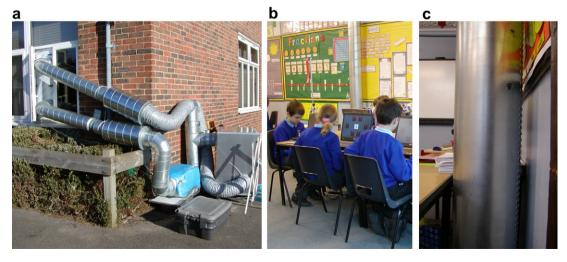
Fig. 1. Exterior fan of the mobile ventilation system (a); testing area with the measuring trolley in the background (b) and air terminal device (c).
