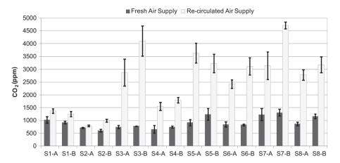
Fig. 2. Mean CO<sub>2</sub> concentrations (±SD) during the computerized performance tests in 16 classrooms at 8 schools. Note: For Schools S1 to S3 no recirculation was carried out; the low ventilation condition was obtained by not changing the windows openings unless the teachers decided so.
