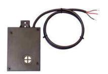
eSENSE™ Slim is used to measure indoor air carbon dioxide concentration. This product is an ultra-compact transmitter intended for factory mounting for both wall and duct applications with the protection class IP50. A 300 mm long cable connected to the PCB makes it possible to place the sensor where mounting is difficult.
