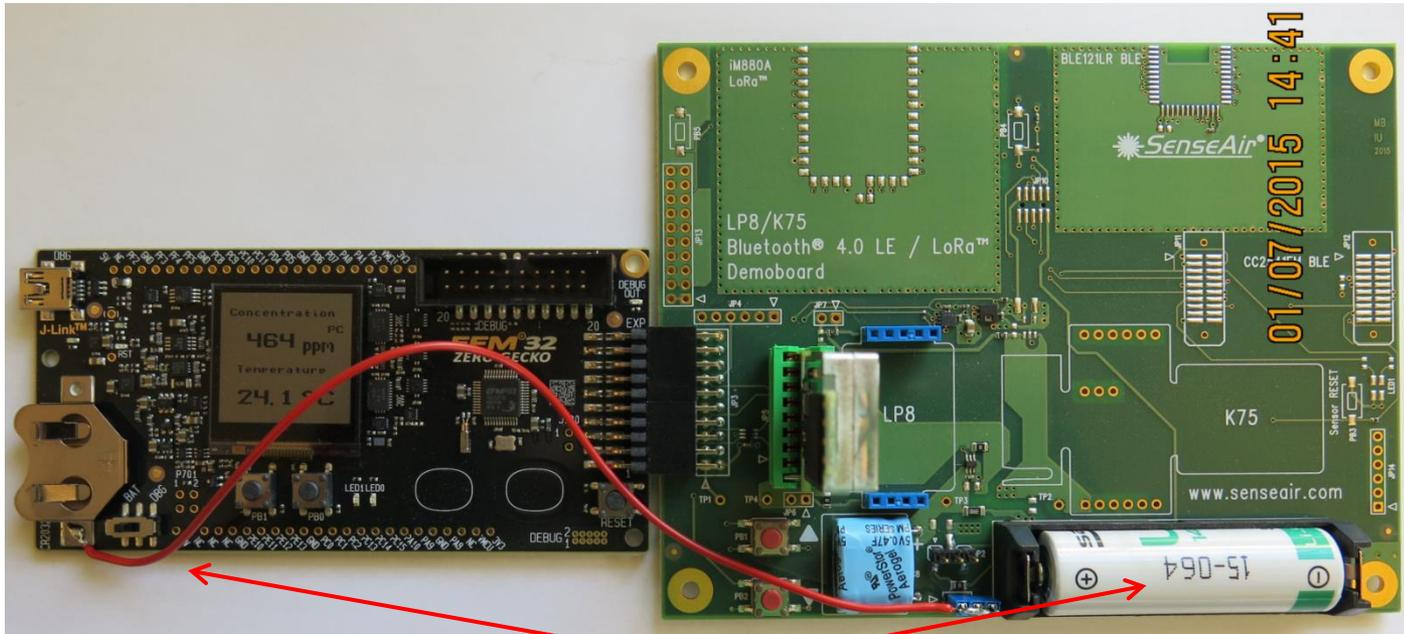
Battery on the Demoboard is used to power EFM32 Starter Kit.
