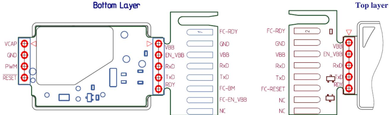
**Note:** VCAP and EN\_VBB are connected to VBB at Factory Connector (if sensor is supplied with Factor Connector).
