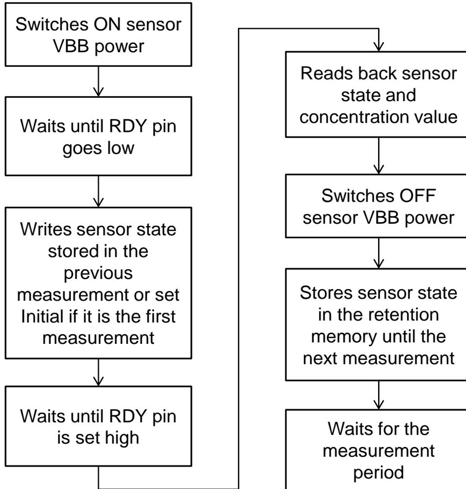
Measurement period of the sensor is determined by customer host system and may vary without degrading measurement accuracy. Minimum allowed measurement period is 16 seconds (below 16 seconds accuracy is not guaranteed).
